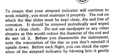
from at least 6 inches away (this reduces the possibility of blowing moist air into it). One last suggestion — check your airspeed indicator frequently for stowaways. On several occasions spiders and other creepy-crawly-critters have climbed through the inlet port with the intention of taking up residence. Needless to say, a bug which weighs as much as the disc can influence the reading considerably if he decides to go for a ride.
