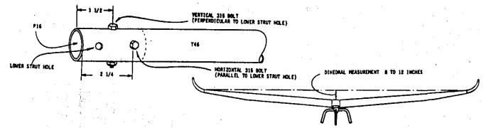
If it is necessary to reposition your P16 plugs, it should be possible to do so without having to scrap either the strut or the plug. Wherever possible, use existing holes in the strut. Rotate the P16 and drill new holes in it as necessary. Make sure the center of the lower strut hole is at least 1/2 inch from the end of the strut.
