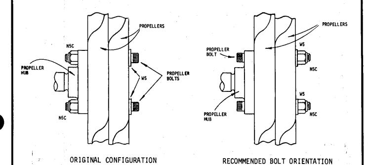
This requires drilling out the holes in the propeller hub to 5/16 inches diameter, and allows the part of the bolt which goes through the hub (where the stress is highest) to be the full diameter. As originally configured, the bolts were threaded into the propeller hub.
