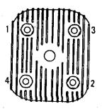
When re-torquing the nuts, they should be torqued to 17 foot-pounds. If a head has been removed, or the nuts are very loose, tighten all the nuts to 5 foot pounds each (using the sequence above), then to 10 foot pounds, then to 17 foot pounds.
