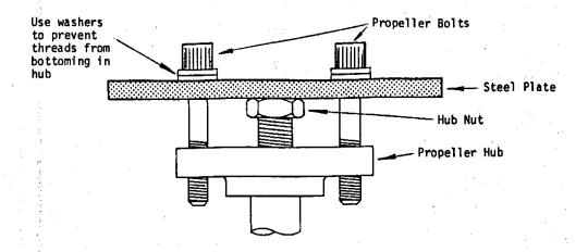
When drilling the holes to 5/16" diameter, make sure the drill is perpendicular to the face of the hub. Make sure you put the bolts in the hub before you install the hub on the crankshaft.
