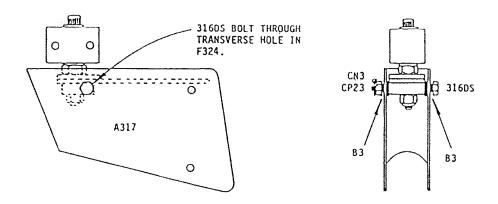
Install the S1205 spacer with a 316 bolt (below the F322 leaf spring). Install the G312 stop and rivet in place as shown to retain the spring. Note that the spring should not be clamped by G312 (about 1/16 of an inch play is acceptable).
