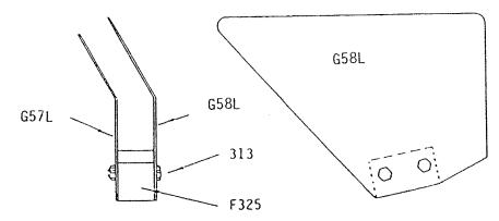
2.4 Remove the F325 tailwheel mount blocks from the aircraft. Grease the SCS250 pivot bolt and assemble the two tailwheel spring and pivot assemblies as shown. The nut between F325 and F323 should be adjusted so that F325 will rotate freely on the bolt but there is little or no
