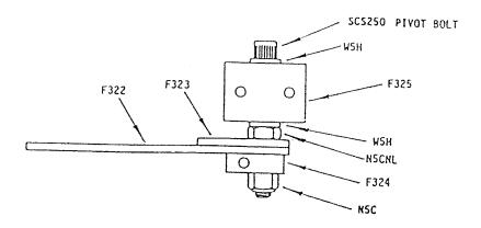
2.5 Fit each spring and pivot assembly into a tailwheel pant (A317) as shown. Adjust the CN3 so that A317 will move freely, and pin the nut with a CP23 cotter pin. Make a left and right assembly by inserting the two 316DS bolts in opposite directions. (The left assembly is shown in the figure).
