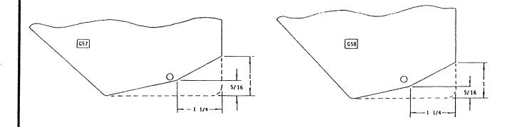
2.2 Drill the 3/16 inch mounting holes in G57 and G58 as shown.
