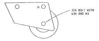
2.8 Reinstall the F325 mount blocks on the aircraft. Check that the tailwheel assembly rotates freely on its pivot bolt. Press down on the top of the tail and check that the tailwheel springs deflect.
